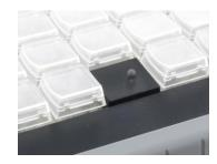
1. Using a pair of needle-nosed pliers with cross hatched jaws, grip the cross of the stem of the plunger and pull straight upward.
