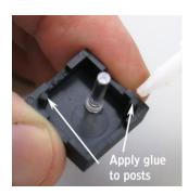
3. Press the blocker firmly into place and hold or clamp it down until the glue sets.
